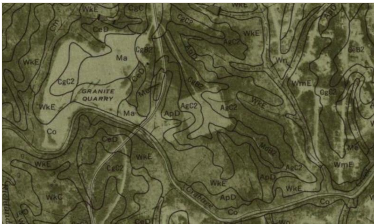
Figure 4. Excerpt from Sheet 38 from the Wake County Soil Survey (1970), showing the site – north of Crabtree Creek and south of the cleared square of the radio towers – as Wake E (described as less than 10 to 20 inches of soil over bedrock, at slopes up to 30 degrees). The asphalt plant site also shows east of Duraleigh Road, north of the creek.
